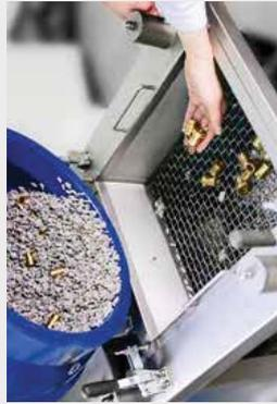
Separating units facilitate separation of mass finished workpieces. Manual separating is time consuming and reduce the efficiency of the process. Automatic separation integrated into mass finishing machine is a great solution for large scale production of small workpieces, which are difficult to be separated manually. Workpieces are separated from the media on the vibrating screen. Automatic separating units are suitable for machines with capacities starting from 18 litres.
